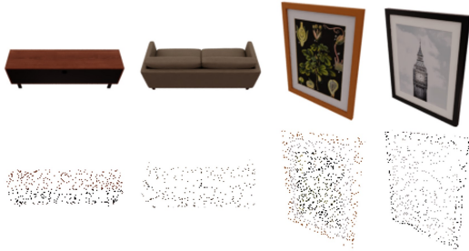
Figure 3. The ambiguity caused by sparsity. The original meshes are shown in the top row and the sampled point clouds are correspondingly shown in the bottom. Meshes of different shapes may be sampled into similar point clouds. And for those similarly shaped meshes, there may be loss of texture details when sampled.
